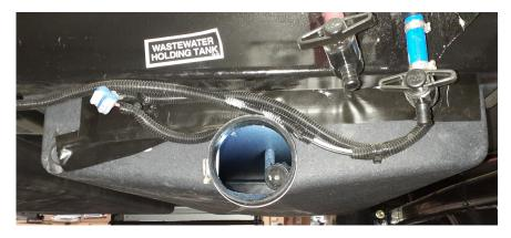
With the inlet assy. removed look inside the tank the white PVC Pipes should only be about 1" or so into tank from top of the tank rubber grommets. If they are to long like the pic. they will need cut off at the desired length of approximately 1" or drill a 5/8" hole with a spade bit ans extension. See pic below:
