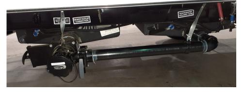
Remove the slicer valve bolts/nuts x4 on the Waste tank assy. and then loosen the hose clamp that is around the ABS reducer inlet on the grey tank assy. remove hanger strap and pull out the plumbing assy. from the grey tank assy.
