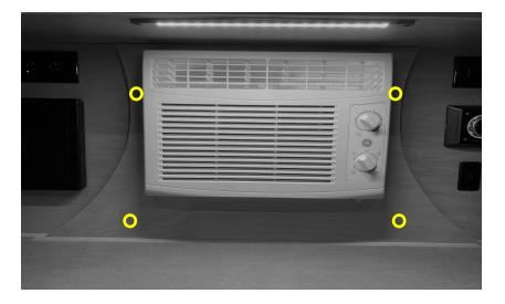
Remove the AC coverboard by peeling off the decorative stickers and removing four (4) 1" mounting screws.
