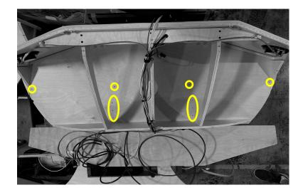
Using a 90-degree drill or adapter, remove (10) 1-1/4 inch black wood screws from the middle cabinet deck. This detaches the Upper Assembly from the Lower Assembly
