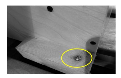
On both sides of the Lower Assembly's AC compartment, are two 2x2 blocks. At present, a single #10 screw goes through each block, through the fiberglass floor, and into the aluminum frame. Remove these screws and discard.
