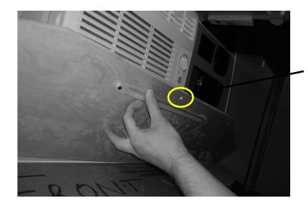
Remove the 1/4" cover board from underneath the front overhang. The back of the coverboard slides into a groove; the front is attached with a single screw
