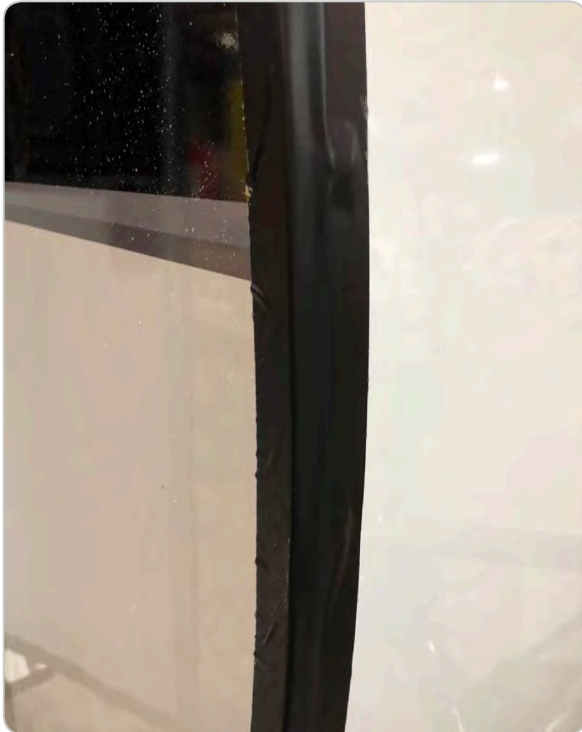
Under Trim Piece. Sealed with EternaBond tape. EternaBond tape is heavy-duty sealing tape used most commonly for military applications.
