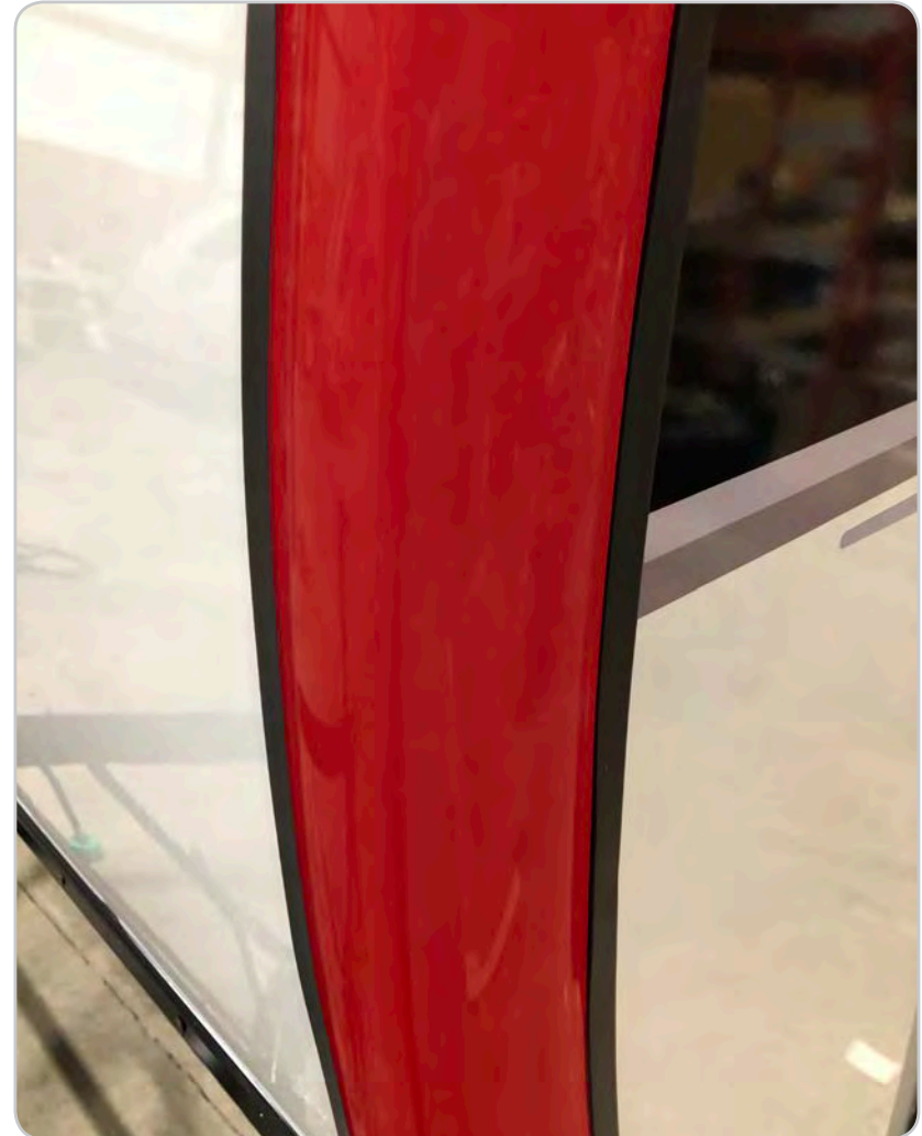
Finished Little Guy Max Trim Piece with EternaBond tape underneath.
