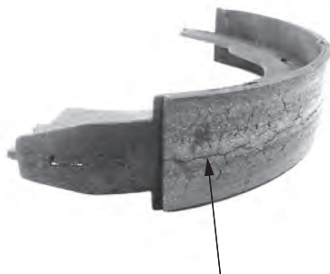
Acceptable Hairline Cracks
